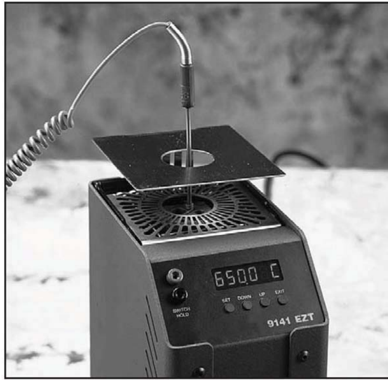
Figure 1 Heat shield installed on 9141 calibrator
